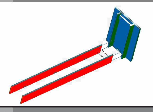
Align Seat Braces with the Side as shown with the cutouts facing in and holes in the end aligned with the threaded holes of the Side Assembly. Insert 7/8" Black bolts and finger tighten to attach.
